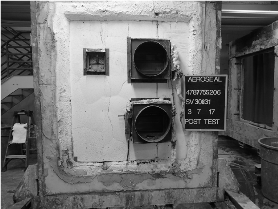
EXPOSED SIDE OF TEST ASSEMBLY AFTER TEST
