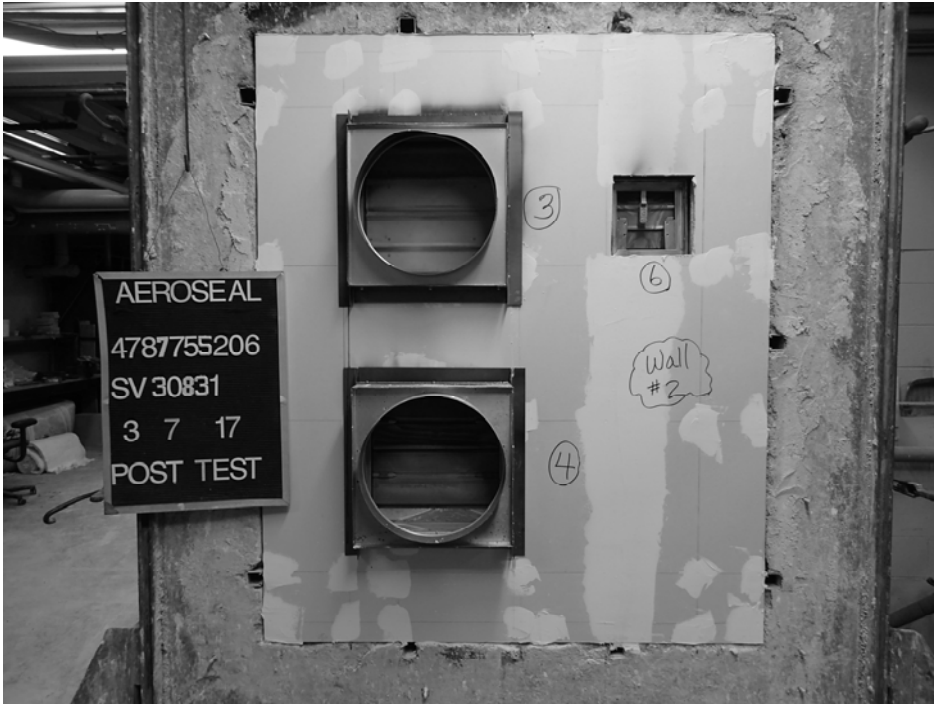
UNEXPOSED SIDE OF TEST ASSEMBLY AFTER TEST
