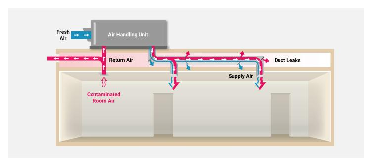
**How Leaky Ductwork Impacts IAQ:** Leaks in the supply and return ductwork impacts IAQ. First by reducing the dilution of contaminated indoor air and then by exhausting less of this diluted air from the building.
