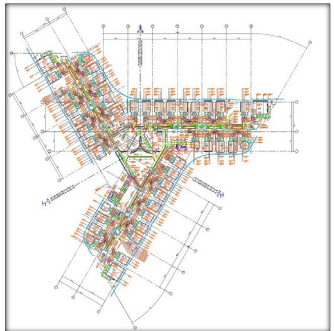
Figure 2: Hotel HVAC Ducting Layout.
